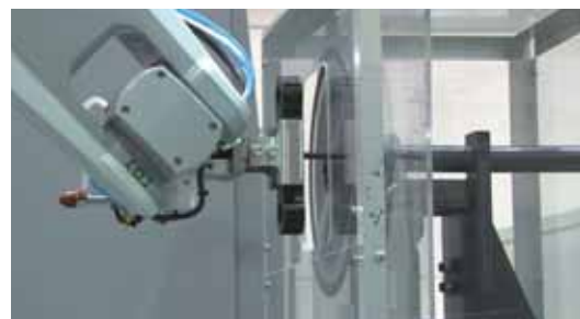
Sprue cutting of a CF RTP molded item
